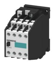
Contactor relay, 53E, DIN EN 50011, 5NO + 3NC, screw terminal AC operation 120 V AC 60 Hz/110 V AC 50 Hz
