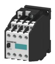
Contactor relay, 53E, DIN EN 50011, 5NO + 3NC, screw terminal AC operation 110V AC 50/60Hz
