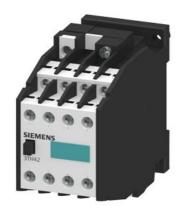
Contactor relay, 44E, DIN EN 50011, 4NO + 4NC, screw terminal AC operation 230/220 V AC 50 Hz, 276/264V 60Hz
