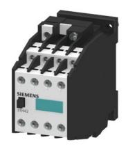
Contactor relay, 44E, DIN EN 50011, 4NO + 4NC, screw terminal AC operation 220 V AC 50/60 Hz
