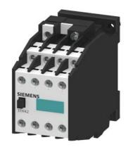
Contactor relay, 44E, DIN EN 50011, 4NO + 4NC, screw terminal AC operation 110V AC 50/60Hz
