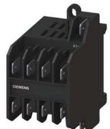
power relay, AC-3, 8.4 A, 4 kW / 400 V, 3-pole, 110 V AC, 45-450 Hz, auxiliary contacts: 1 NO, flat connector 6.3 x 0.8 mm
