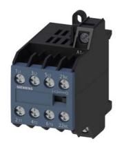
power relay, AC-3, 8.4 A, 4 kW / 400 V, 3-pole, 24 V DC, auxiliary contacts: 1 NC, screw terminal
