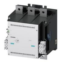
Contactor, Size 14, 3-pole, AC-3, 450 kW, 400/380 V (690 V) Auxiliary switch 44 (4NO+4NC) AC operation 500...600 V AC 50/60 Hz
