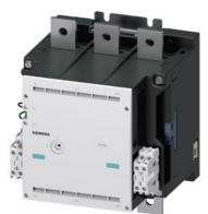
vacuum contactor AC-3e 630 A, 335 kW / 400 V, AC-3 820 A, 450 kW / 400 V, Ue 690 V, 3-pole, Uc: 380-460 V AC(50/60 Hz) drive: conventional auxiliary contacts 4 NO + 4 NC main circuit: busbar control and auxiliary circuit: screw terminal
