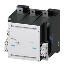
vacuum contactor AC-3e/AC-3 630 A, 335 kW / 400 V, Ue 690 V, 3-pole, Uc: 380-460 V AC(50/60 Hz) drive: conventional auxiliary contacts 4 NO + 4 NC main circuit: busbar control and auxiliary circuit: screw terminal
