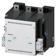
vacuum contactor AC-3e/AC-3 630 A, 335 kW / 400 V, Ue 690 V, 3-pole, Uc: 230-276 V AC(50/60 Hz) drive: conventional auxiliary contacts 4 NO + 4 NC main circuit: busbar control and auxiliary circuit: screw terminal
