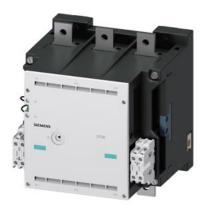
vacuum contactor AC-3e/AC-3 630 A, 335 kW / 400 V, Ue 690 V, 3-pole, Uc: 200-240 V AC(50/60 Hz) drive: conventional auxiliary contacts 4 NO + 4 NC main circuit: busbar control and auxiliary circuit: screw terminal
