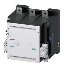
vacuum contactor AC-3e/AC-3 630 A, 335 kW / 400 V, Ue 690 V, 3-pole, Uc: 110-132 V AC(50/60 Hz) drive: conventional auxiliary contacts 4 NO + 4 NC main circuit: busbar control and auxiliary circuit: screw terminal without overvoltage damping in main circuit
