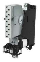
Traction contactor 1-pole 400 A 4 NO+4 NC 24 V DC with integrated varistor
