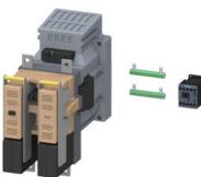
Contactor, size 12, 2-pole, DC-3 and 5, 400 A at 750 V Auxiliary contacts 21 (2NO + 1NC) 24V DC DC operation with varistor and series resistor Operating range 0.7 to 1.25 x US DC operation
