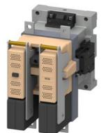
Contactor size 12, 2-pole DC-3 and 5, 400 A Auxiliary switch 22 (2 NO + 2 NC) Direct current operation 120 V AC 60 Hz/100 V AC 50 Hz
