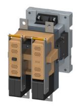
Contactor, Size 8, 2-pole, DC-3 and 5, 220 A Auxiliary switch 22 (2 NO + 2 NC) 230V AC 50Hz, 277 V 60 Hz AC operation AC operation
