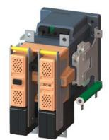
Contactor, Size 4, 2-pole, DC-3 and 5, 75 A at 750 V Auxiliary contacts 21 (2NO + 1NC) 36 V DC DC operation with varistor and series resistor Operating range 0.7 to 1.25 x US
