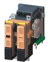
Contactor, Size 4, 2-pole, DC-3 and 5, 75 A at 750 V Auxiliary contacts 21 (2NO + 1NC) 110V DC DC operation with varistor and series resistor Operating range 0.7 to 1.25 x US
