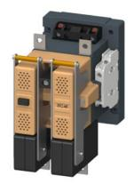
Contactor, Size 4, 2-pole, DC-3 and 5, 75 A Auxiliary switch 22 (2 NO + 2 NC) 240 V AC 50 Hz/288 V AC 60 Hz AC operation
