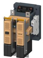
Contactor size 4, 2-pole DC-3 and 5, 75 A Auxiliary switch 22 (2 NO + 2 NC) Alternating current operation 230 V AC 60 Hz/192 V AC 50 Hz
