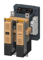
Contactor size 4, 2-pole DC-3 and 5, 75 A Auxiliary switch 22 (2 NO + 2 NC) Alternating current operation 120 V AC 60 Hz/110 V AC 50 Hz
