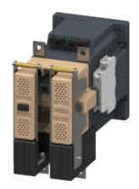
Contactor, Size 4, 2-pole, DC-3 and 5, 75 A Auxiliary switch 22 (2 NO + 2 NC) 220V DC DC operation
