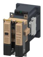
Contactor, Size 4, 2-pole, DC-3 and 5, 75 A Auxiliary switch 22 (2 NO + 2 NC) 110V DC DC operation
