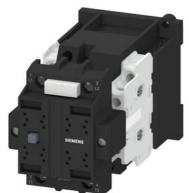
Contactor, Size 2, 2-pole, DC-3 and 5, 32 A Auxiliary switch 22 (2 NO + 2 NC) 24V DC DC operation with integrated varistor
