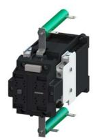
Contactor size 2, 2-pole for railway applications DC-3 and 5, 7.5 A at 750 V Auxiliary contacts 21 (2 NO + 1 NC) Operating range 0.7 to 1.25 x US connected to varistor DC magnet system 24 V DC Upright mounting position
