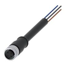
Connection cable with M12 socket 4-pole, straight and free cable end 5 m long. For connection for position switch 3SE52, round magnetic switch 3SE66 or 8WD46 with 4-pole M12 plug.
