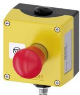
Enclosure for command devices, 22 mm, round, enclosure material metal, Enclosure top part yellow, 1 control point metal, A=Emergency stop mushroom pushbutton red, 40 mm, rotate-to-unlatch, 2 NC, spring-loaded terminal, floor mounting, silver label, black font, with graphic symbol: Emergency stop, M12 connector (5-pin) bottom, insulated reserve conductors Label glued in
