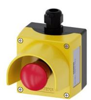
AS-Interface enclosure for command devices 22 mm, round, Enclosure material metal, Enclosure top part yellow, with protective collar, 1 control point metal, A=EMERGENCY STOP mushroom pushbutton red, 40 mm, rotate-to-unlatch, 1 NC, 1 NC, spring-type terminal, floor mounting, AS-i shaped cable Direct entry top/right
