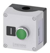
Enclosure for command devices, 22 mm, round, Enclosure material metal, enclosure top part gray, 1 control point metal, A=Pushbutton green, 1 NO, screw terminal, floor mounting, label: I, 1xM20 each on top and bottom, Label enclosed
