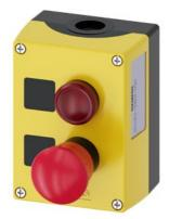
Enclosure for command devices, 22 mm, round, Enclosure material plastic, Enclosure top part yellow, 2 control points plastic, B=Indicator light red, LED 24 V, screw terminal, label without inscription, A=Emergency stop 40 mm rotate-tounlatch, label without inscription, 1 NO, 1 NC, 1 NC, screw terminal, floor mounting, 1xM20 each on top and bottom, Labels enclosed
