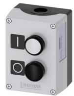
Enclosure for command devices, 22 mm, round, Enclosure material plastic, enclosure top part gray, 2 control points plastic, Recess for labels, B=Pushbutton white, label: I, 1 NO, screw terminal, A=Pushbutton black label: O 1 NC, screw terminal, floor mounting, Labels enclosed
