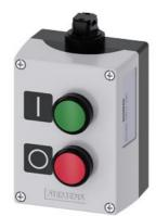
AS-Interface enclosure for command devices, 22 mm, round, Enclosure material plastic, enclosure top part gray, 2 control points plastic, Recess for labels, B=Pushbutton green, label: I, 1 NO, spring-type terminal, A=Pushbutton red, label: O, 1 NC, spring-type terminal, floor mounting, Insulation displacement system on top, Labels enclosed
