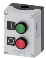
Enclosure for command devices, 22 mm, round, Enclosure material plastic, enclosure top part gray, 2 control points plastic, B=Pushbutton green, label: I, 1 NO, screw terminal, A=Pushbutton red, label: O, 1 NC, screw terminal, floor mounting, 1xM20 each on top and bottom, Labels enclosed
