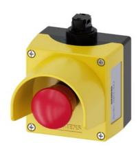
AS-Interface enclosure for command devices 22 mm, round, Enclosure material plastic, Enclosure top part yellow, with protective collar, 1 control point plastic, A=EMERGENCY STOP mushroom pushbutton red, 40 mm, rotate-to-unlatch, 1 NC, 1 NC, spring-type terminal, floor mounting, Insulation displacement system on top
