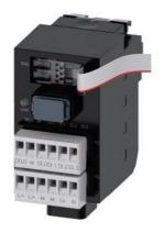
SIRIUS ACT with PROFINET: standard interface module with extended inputs and outputs 24 V DC, screw terminal, front plate mounting, 1 to 20 terminal modules connectable, with additional 1 DQ + 4 DI + 1 AI
