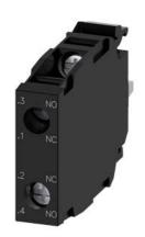
Contact module with 2 contact elements, 1 NO+1 NC, gold-plated contacts, screw terminal, for front plate mounting  $\,$
