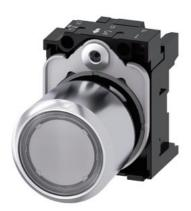
Pushbutton, compact, with extended stroke (12 mm), 22 mm, round, Metal, clear, pushbutton, flat, momentary contact type, with holder, Z=50-unit packaging
