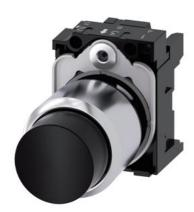
Pushbutton, compact, with extended stroke (12 mm), 22 mm, round, Metal, black, pushbutton, high, momentary contact type, with holder, with laser labeling, inscription or symbol Customer-specific selection with SIRIUS ACT configurator (CIN)
