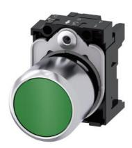
Pushbutton, compact, with extended stroke (12 mm), 22 mm, round, Metal, green, pushbutton, flat, momentary contact type, with holder, with laser labeling, inscription or symbol Customer-specific selection with SIRIUS ACT configurator (CIN)
