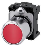
Pushbutton, compact, with extended stroke (12 mm), 22 mm, round, Metal, red, pushbutton, flat, momentary contact type, with holder, with laser labeling, upper case and lower case, always upper case at the beginning of the word
