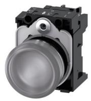
Indicator lights, 22 mm, round, metal, shiny, clear, lens, smooth, with holder, LED module with integrated LED 230 V AC, screw terminal
