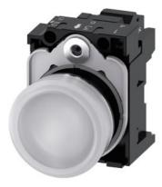
Indicator lights, 22 mm, round, Metal, shiny, white, lens, smooth, with holder, LED module with integrated LED 230 V AC, spring-type terminal, with laser labeling, inscription or symbol Customer-specific selection with SIRIUS ACT configurator (CIN)
