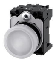
Indicator lights, 22 mm, round, Metal, shiny, white, lens, smooth, with holder, LED module with integrated LED 230 V AC, screw terminal, with laser labeling, upper case and lower case, always upper case at the beginning of the word
