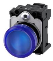
Indicator lights, 22 mm, round, Metal, shiny, blue, lens, smooth, with holder, LED module with integrated LED 230 V AC, spring-type terminal, with laser labeling, symbol number according to, ISO 7000 or IEC 60417
