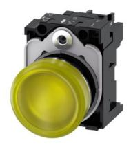
Indicator lights, 22 mm, round, Metal, shiny, yellow, lens, smooth, with holder, LED module with integrated LED 230 V AC, screw terminal, with laser labeling, symbol number according to, ISO 7000 or IEC 60417
