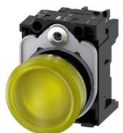
Indicator lights, 22 mm, round, Metal, shiny, yellow, lens, smooth, with holder, LED module with integrated LED 230 V AC, screw terminal, with laser labeling, upper case
