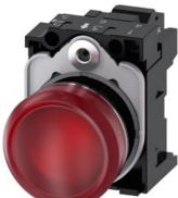
Indicator lights, 22 mm, round, metal, shiny, red, lens, smooth, with holder, LED module with integrated LED 230 V AC, spring-type terminal, Z=20-unit packaging
