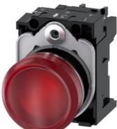
Indicator lights, 22 mm, round, metal, shiny, red, lens, smooth, with holder, LED module with integrated LED 230 V AC, screw terminal, Z=20-unit packaging
