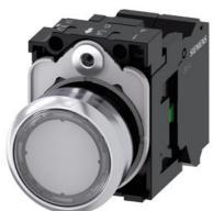
Illuminated pushbutton, 22 mm, round, metal, shiny, transparent, pushbutton, flat, momentary contact type, with holder, 1 NO, LED module with integrated LED 230 V AC, Spring-type terminal
